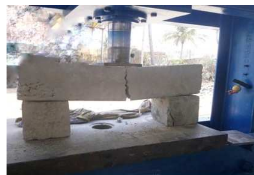
Fig 3 Flexural Strength Testing of Beam
