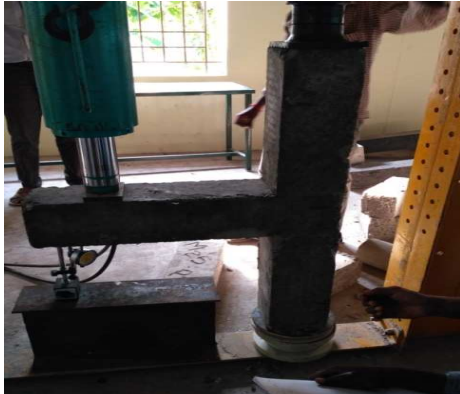
Fig 4 Test on T Beam
