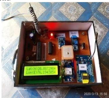
Fig 8: Black Box system connection
