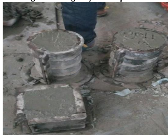
Fig 3.1 Casting of cylinder specimen
