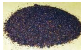
Fig 2.1 Unprocessed foundry sand
