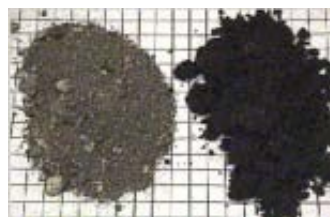
Fig 2.2 Green sands from a gray iron foundry
