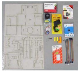
FIGURE 3: Cardboard TJBOT With its parts
