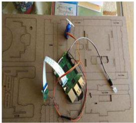
FIGURE 2: TJBOT parts which includes LED light, USB Microphone, Camera, Servo Motor
