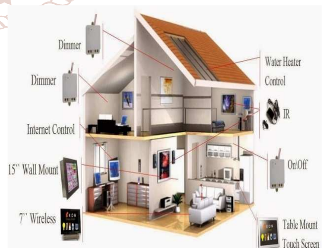
Fig 1.1 Home with an Automated System
