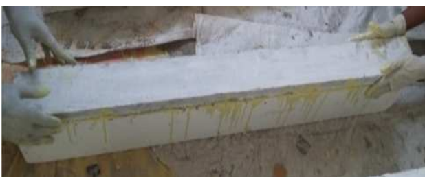
Fig. 4.6 Strengthened RC beam
