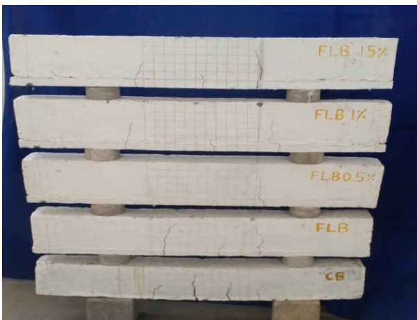
Fig 5.7 Crack patterns of tested specimens
