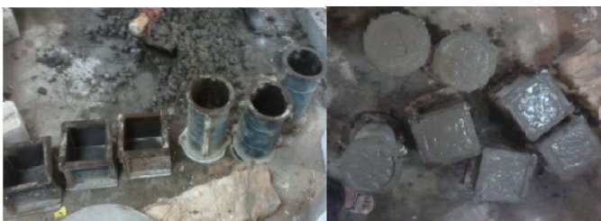
Figure 3.1 Casting of cube and cylinder specimens.
