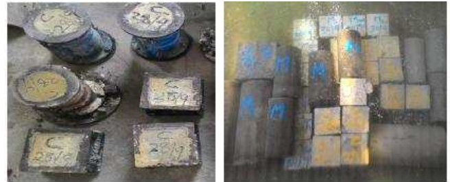
Figure.3.3 Casting and Curing of Specimens
