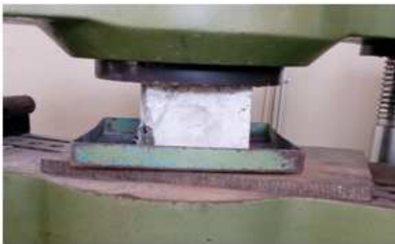
Figure 4.1 Compression Strength Test
