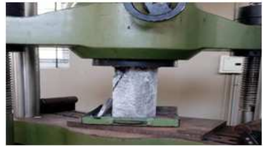
Figure 4.4 Split Tensile Strength Test
