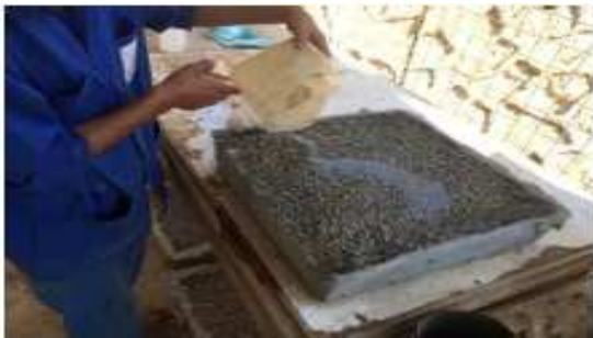
Figure 3: Pouring Polyester for Slab Specimen
