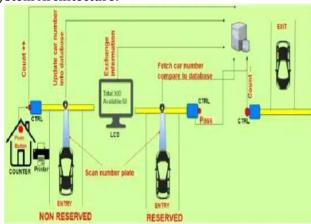
The System Architecture shows the working of the intelligent parking system, In this there will be diverse entryway for the reserved parking and no reserved parking for saving the parking spot the user should have the application of the intelligent parking, the structure where the user will save its place in the stopping station for stopping by paying the charge through on the web.
