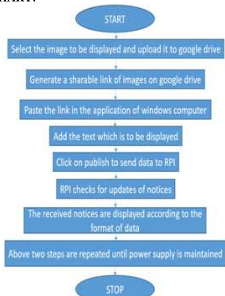
Figure5: system Diagram of Proposed System
