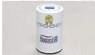
(b) RandonEye(RD200) Radon concentration meter
