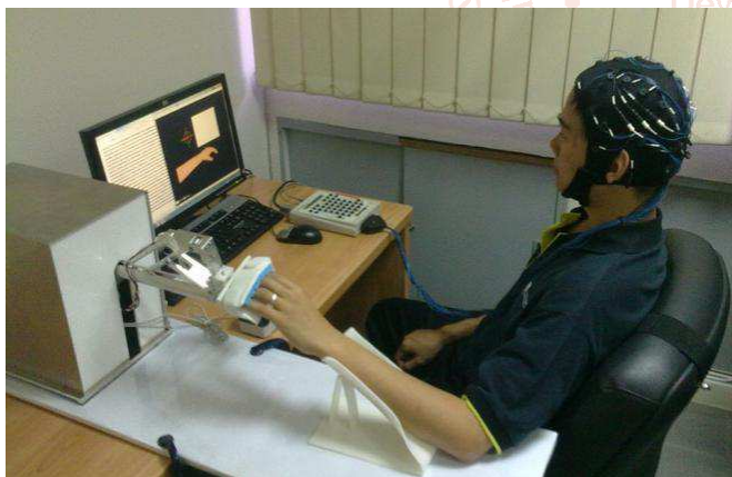
Fig.1. Experimental setup to collect EEG data from passive movement of the left hand
