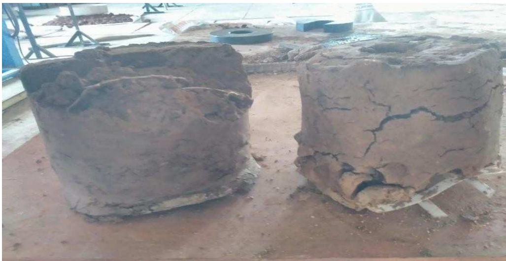
Laboratory Experiment WITH FIBER in CBR Mould
