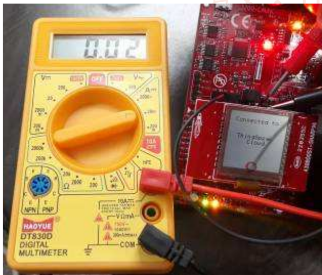
Figure8: The amount current consuming by the system when connecting with cloud based services
