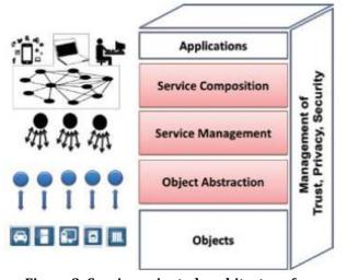
Figure 3: Service-oriented-architecture for a middleware in IoT
