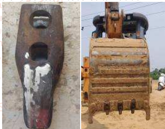
Figure No.1.3: Hardfaced tooth and Field test at Aadhaar hospital, Hisar
