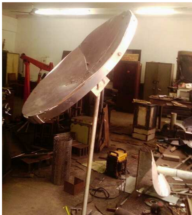
Plate 1.0: Photo of side view of the prototype of reflector dish (without feed)
