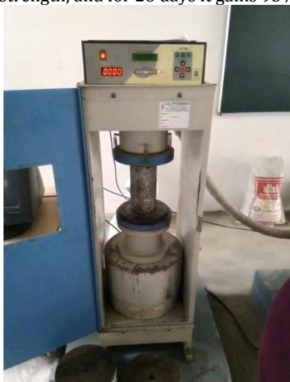
Figure3. Testing of cylinder for Compressive strength
