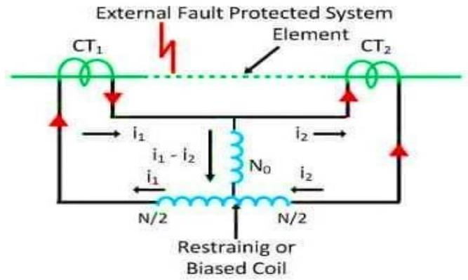
**Figure2. Biased or Percentage Differential Relay**
