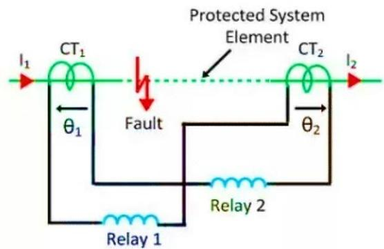
**Figure3. Voltage Balance Differential Relay**
