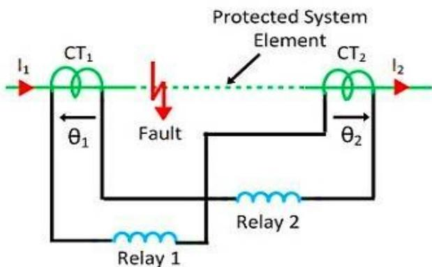
**Figure1. Current Differential Relay**
