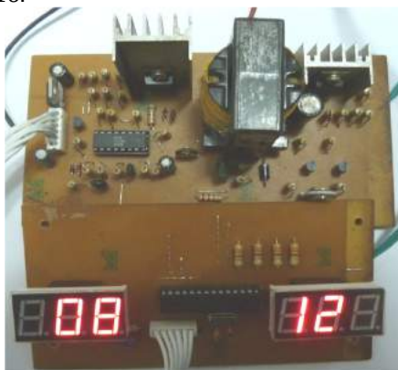
Figure 16 DC to DC Converters in Step-up Converting Mode
