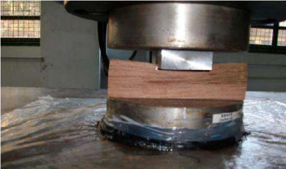
Fig.9 Experimental Set-up of Compression Perpendicular to Grain
