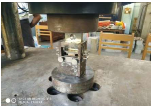
Fig. 11 Experimental Set-up of Shear Parallel to Grain
