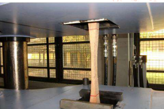
Fig. 10 Experimental Set-up of Tension Parallel to Grain
