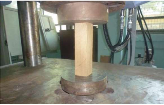
Fig.8 Experimental Set-up of Compression Parallel to Grain
