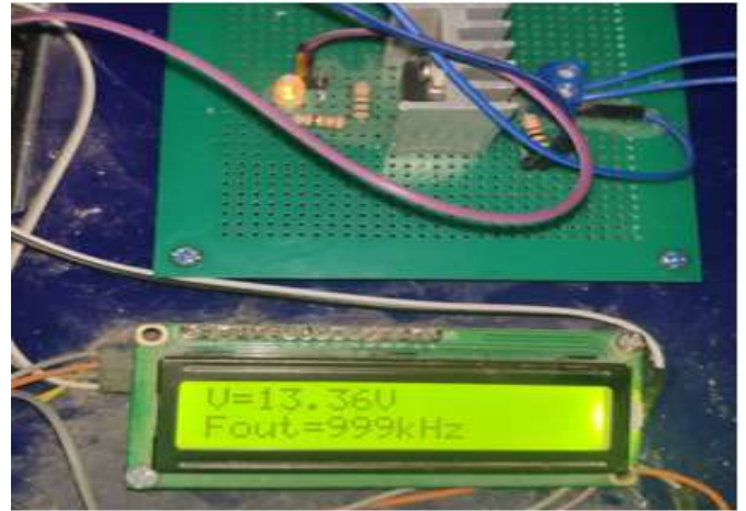
Figure.13 Frequency Generated From Transmitter
