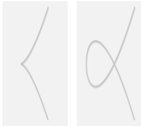
Figure A.2 Types of singularities: on the left, a curve with a cusp ( y^2=x^3 ). On the right, a curve with a self-intersection ( y^2=x^3-3x+2 ). None of them is a valid elliptic curve.
