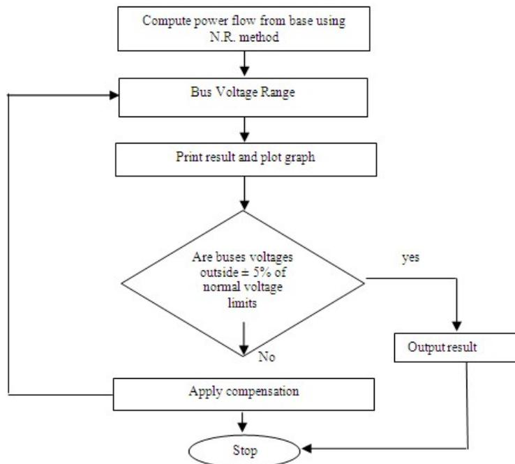
Figure4: Flow Chart for the Analysis of UPFC Compensation Algorithm.
