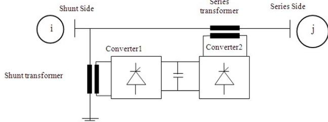
Figure1: Implementation of the UPFC by back to back source converters.
