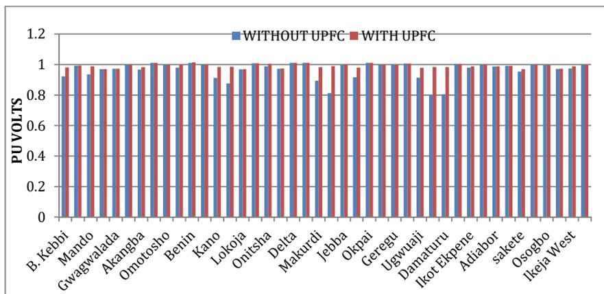
**Figure6: Bar plot of bus voltage with and without UPFC**
