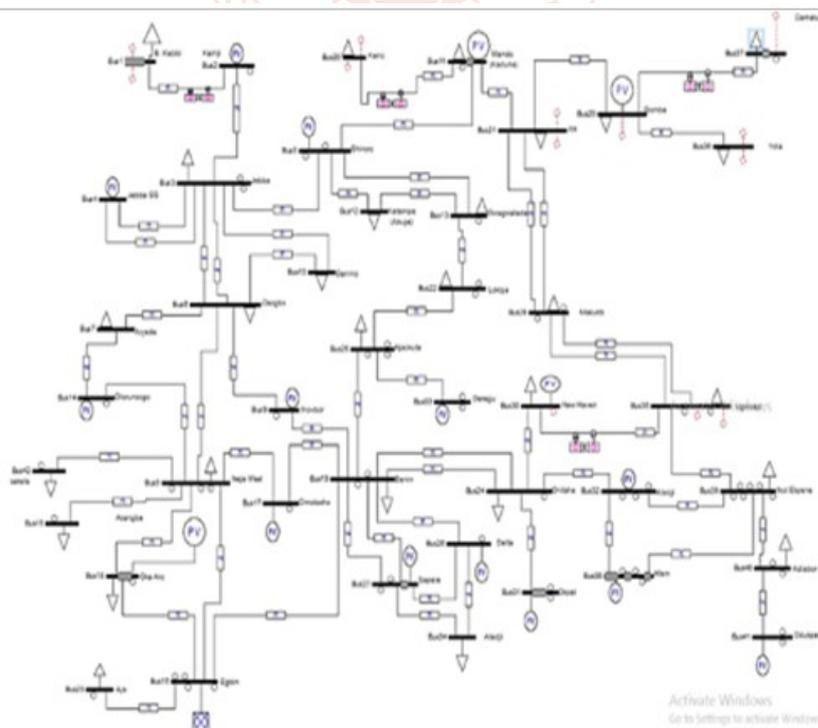
Figure5: Modelled Nigerian 330kV power system on PSAT
