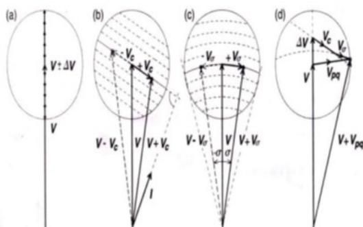
Figure2: Phasor diagram representation of modes of operation of UPFC
