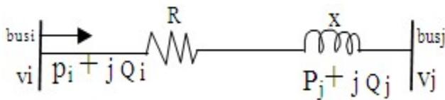
**Figure4: Two bus system line diagram of transmission line**
