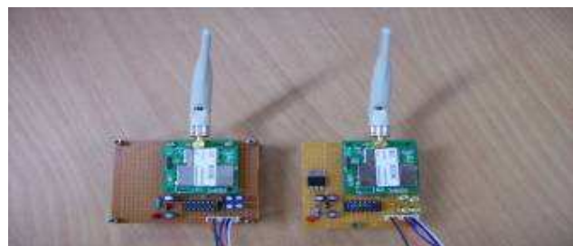
Fig.2 left: ZCM(ZigBee coordinator modem), right : ZED(ZigBee end device)
