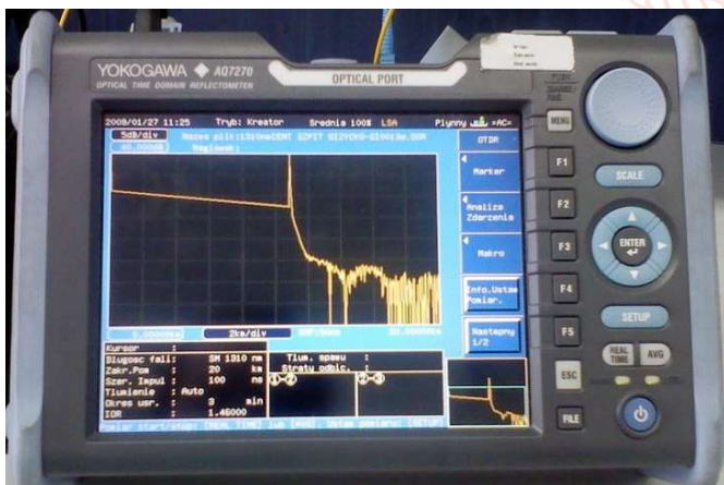
Figure 25 Example of OTDR testing result
