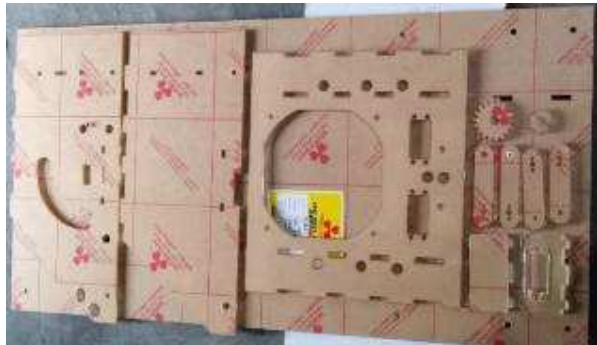
Figure2. The Main Frame of Automatic Car Washing with Fibreboard
