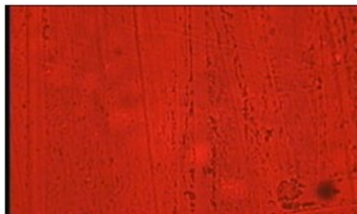
Fig.(7) Photograph of Alpha Track in LR-115 Detector for Cheroot Sample CH-S4
