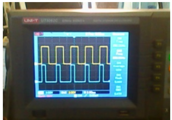
Figure19. 1.992ms and 1.008ms PWM Output of Receiver
