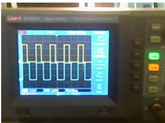
Figure16. 1ms and 2ms PWM Output of Receiver Circuit
