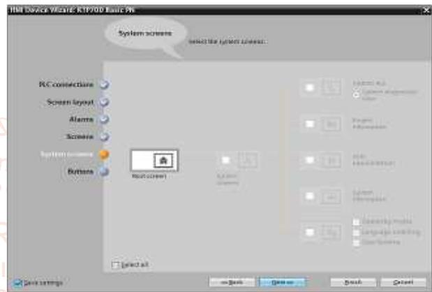
**Figure10 (e). Configure the system screens using the HMI device wizard**
