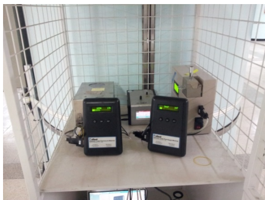
Fig.4. The PM measuring instruments Airstest PM2500 and HCT 4103 installed at a subway station
