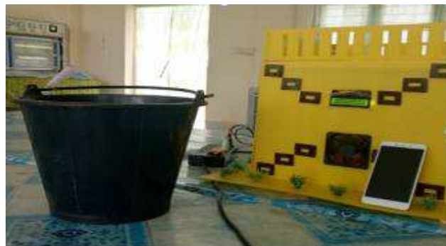
Fig 13: Rotation of Fan with 250rpm between temperature 36°C and 40°C
