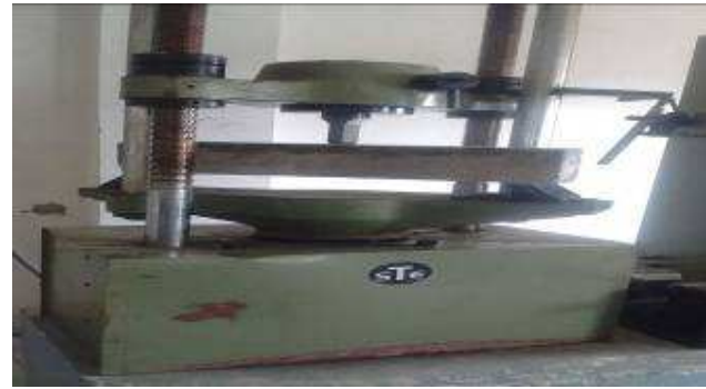
Figure6 Flexural test setup
