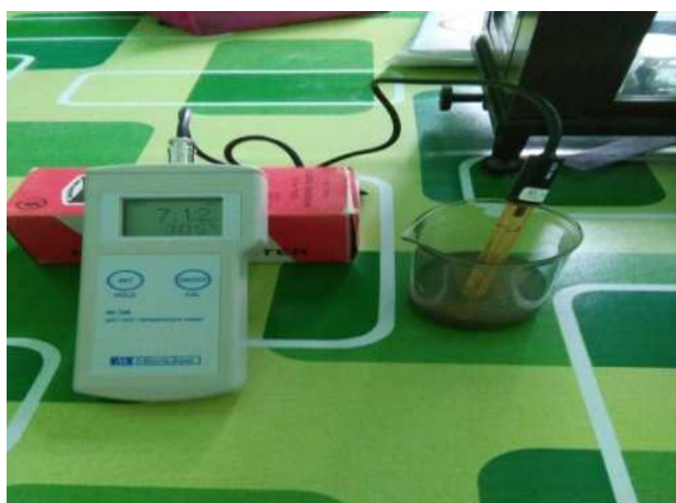
Figure 1: The pH value of eggshells powder with temperature 200°C
