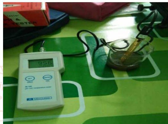
Figure3: The pH value of eggshells powder with temperature 400°C
