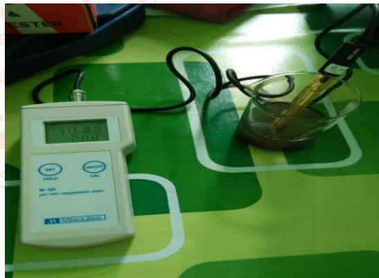
Figure4: The pH value of eggshells powder with temperature 500°C
