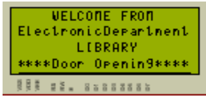
Figure4.2 Door Opened Condition Message on LCD
