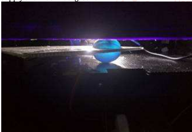
Reading the RGB Values of the Blue Ball with External Light Supply and Black Background
