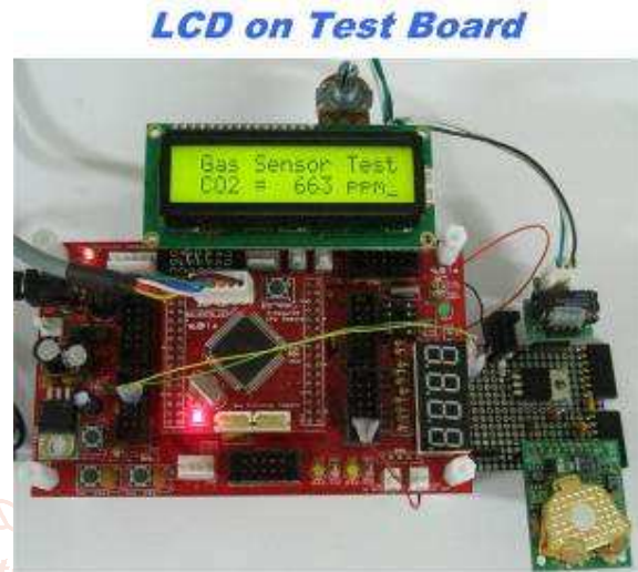
Fig.5. NDIR CO 2 sensor connected to Atmega 128L MCU board
