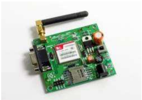
Figure5. SIM900A V4 GSM/GPRS Wireless Extension Module
