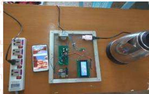
Fig. 5: Electricity Meter Reading System with GSM Module
