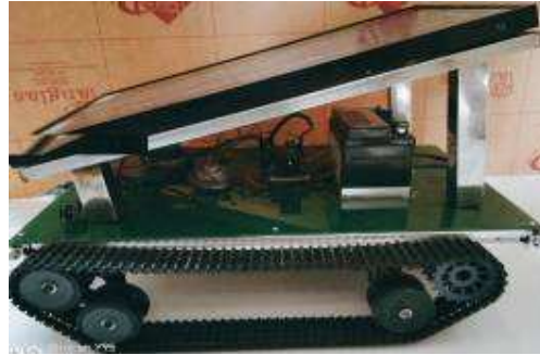
Figure 12(c). Hardware Construction of Solar Based Grass Cutter
