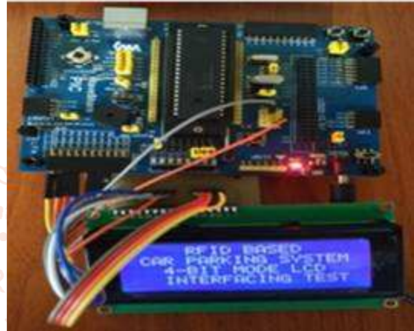
Figure 10. Testing and Result of Interfacing PIC Microcontroller with LCD Display
