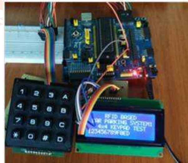
Figure 11. Test and Result of Interfacing 4x4 Matrix Keypad, LCD Display and PIC
