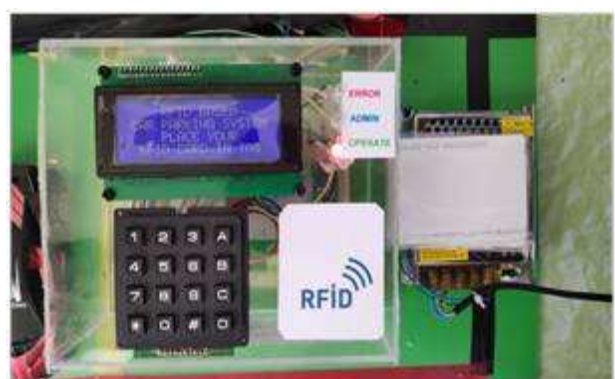
Figure 14. Final Assembly of RFID Based Parking Lot Security System
