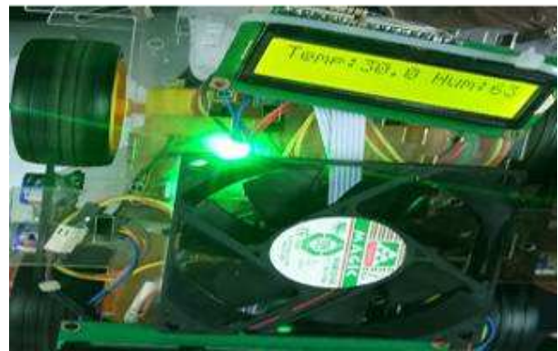
Figure7. Displaying Temperature and Humidity Data on LCD
