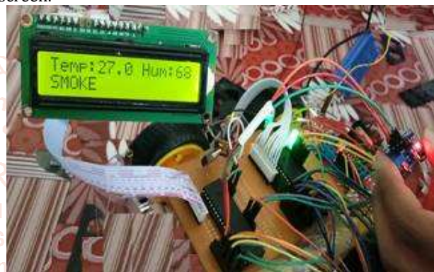
Figure8. Displaying Temperature, Humidity and Smoke Data on LCD
