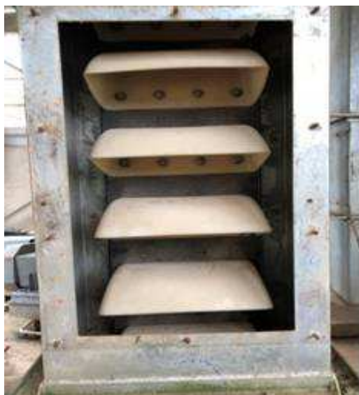
Figure2. Belt and Buckets
