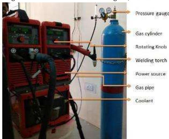
Fig 3.2: Welding Set up
