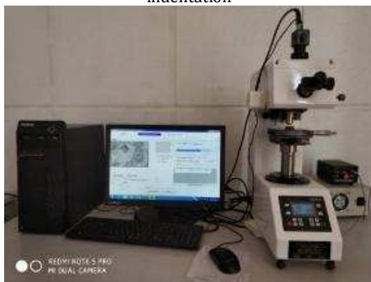
**Fig 3.9: Micro Hardness Testing Setup**
