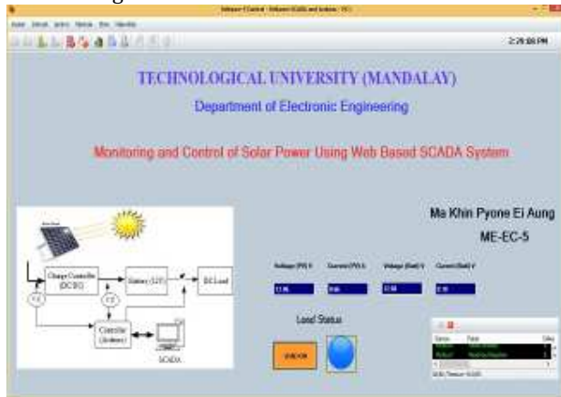
Figure9. User Interface of SCADA System while Running with Load (ON)
