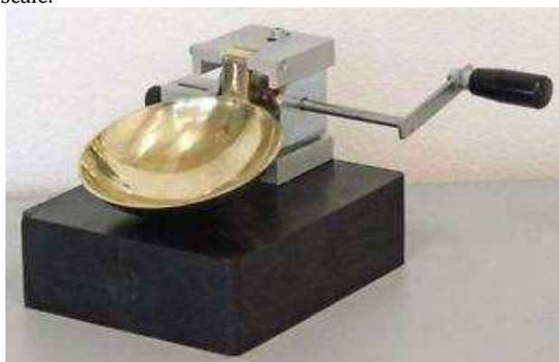
Fig 1: Casagrande's Liquid Limit Device
