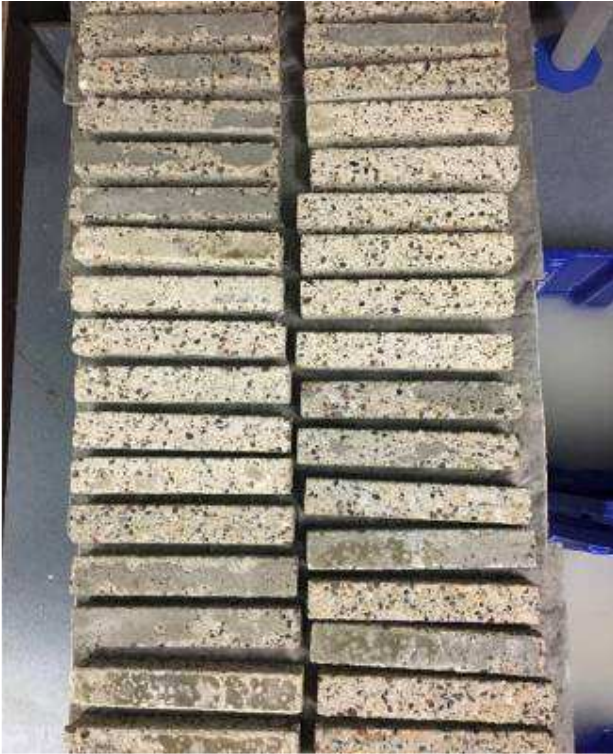
Drying the specimens in laboratory conditions after taking them out of the solution
