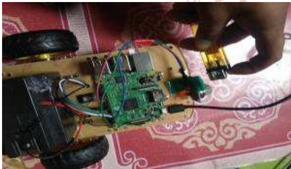
Figure14. The Sensor can't Detect the Gas from Lighter
